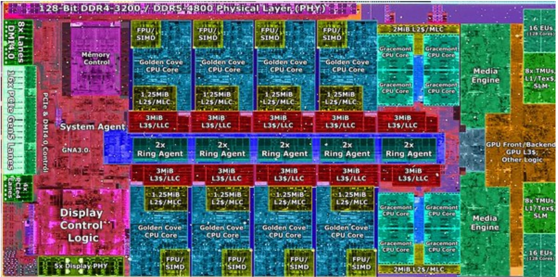
10nm ESF/Intel 7 Alder Lake die shot (~209mm 2 ) from Intel via Andreas Schilling on Twitter: https://twitter.com/aschilling/status/1453391035577495553
