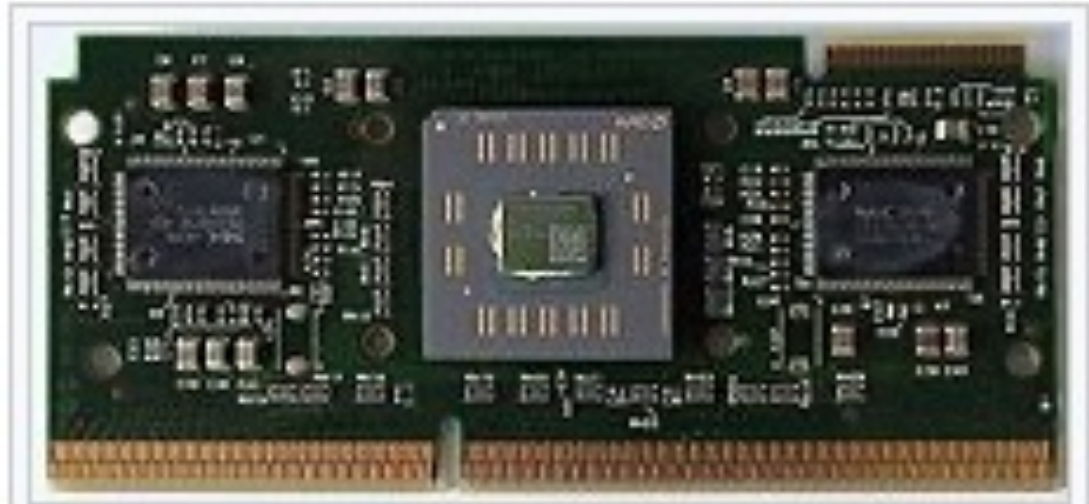
AMD Athlon (early version) – a technically different but fully compatible x86 implementation
