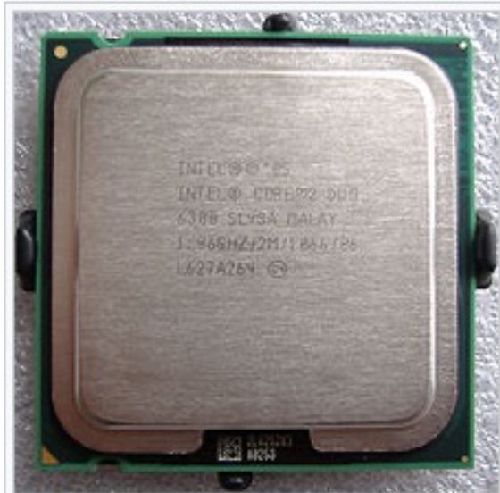
Intel Core 2 Duo – an example of an x86-compatible, 64-bit multicore processor
