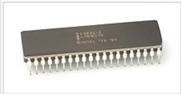
The x86 architectures were based on the Intel 8086 microprocessor chip, initially released in 1978.
