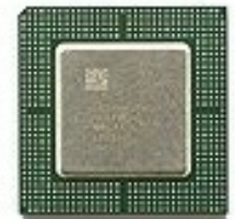
Intel GC80960RN, sSpec: SL3YW, BGA Package
