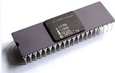
A rare Intel C8086 processor in purple ceramic DIP package with side-brazed pins
